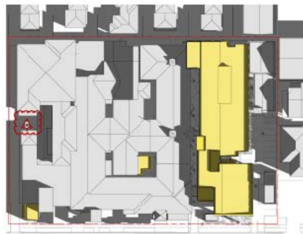
1 PROPOSED SHADOW DIAGRAM JUN 21st 900 Scale 1:500
