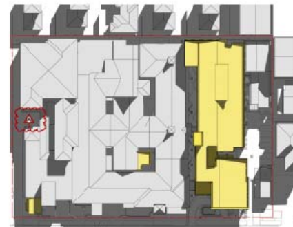
3 PROPOSED SHADOW DIAGRAM JUN 21st 1500 Scale 1:500
